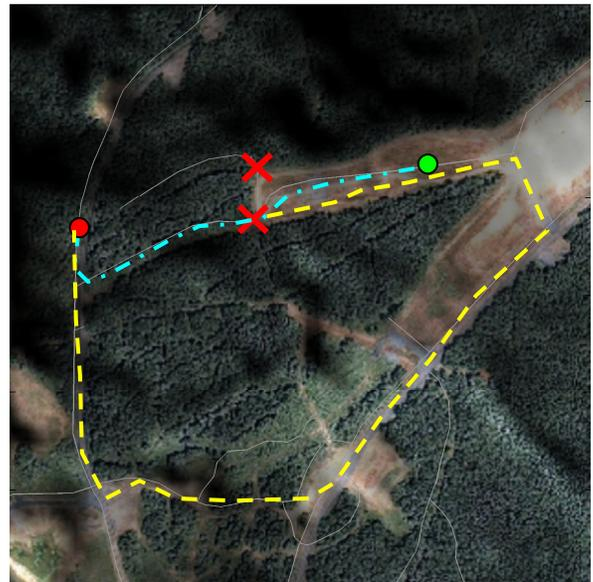
Fig 5. Test scenario for optimizing FCI's performance. The blue line shows the original path, while the yellow line shows one of the possible alternate paths for the robot to follow after the blockages in the main route are detected (red crosses). The area shown is 600x600 meters.
