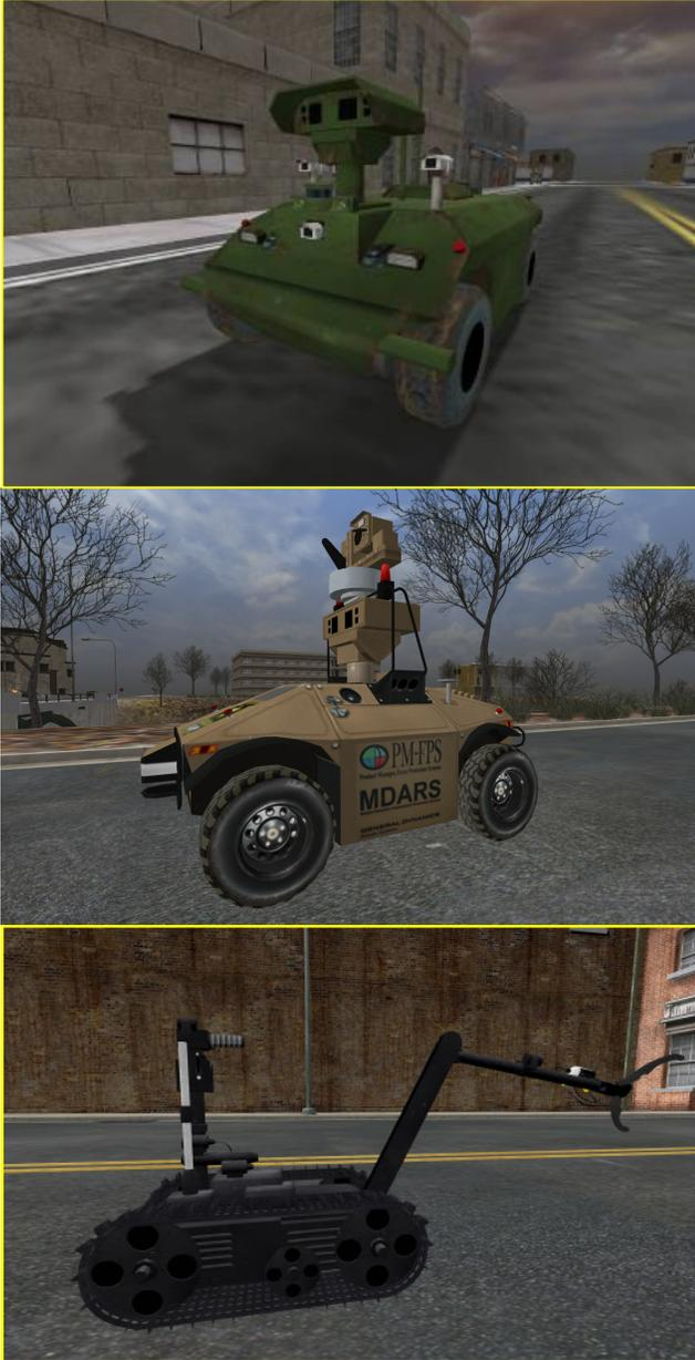
Fig 3. Some of RIVET's simulated platforms: GDRS XUV, MDARS and Talon.
